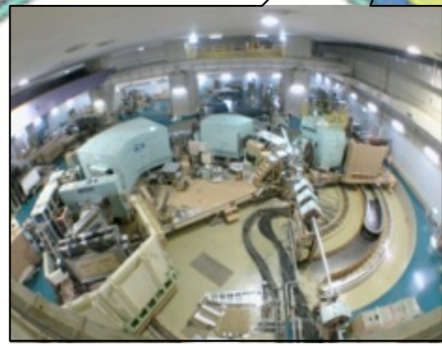
Double arm spectrometer (Grand Raiden & LAS)
