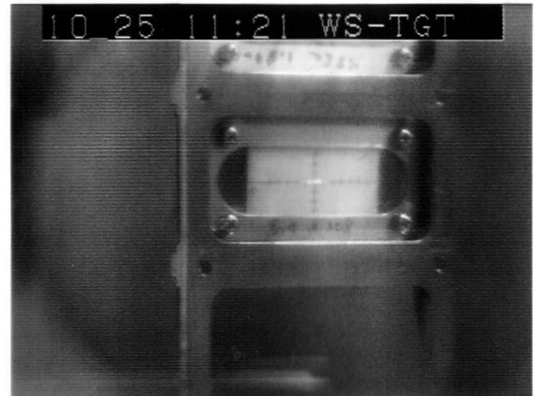
Beam spot in the dispersive mode
