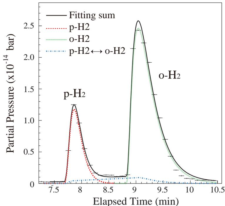
Figure 6.7: The fitting to the data with 2 u/e. Peaks of o-H<sub>2</sub> and p-H<sub>2</sub> are fitted by using Eqn. 6.1. The continuum in the transition region is fitted by using Eqn. 6.4 as shown by the dash-dotted curve.
