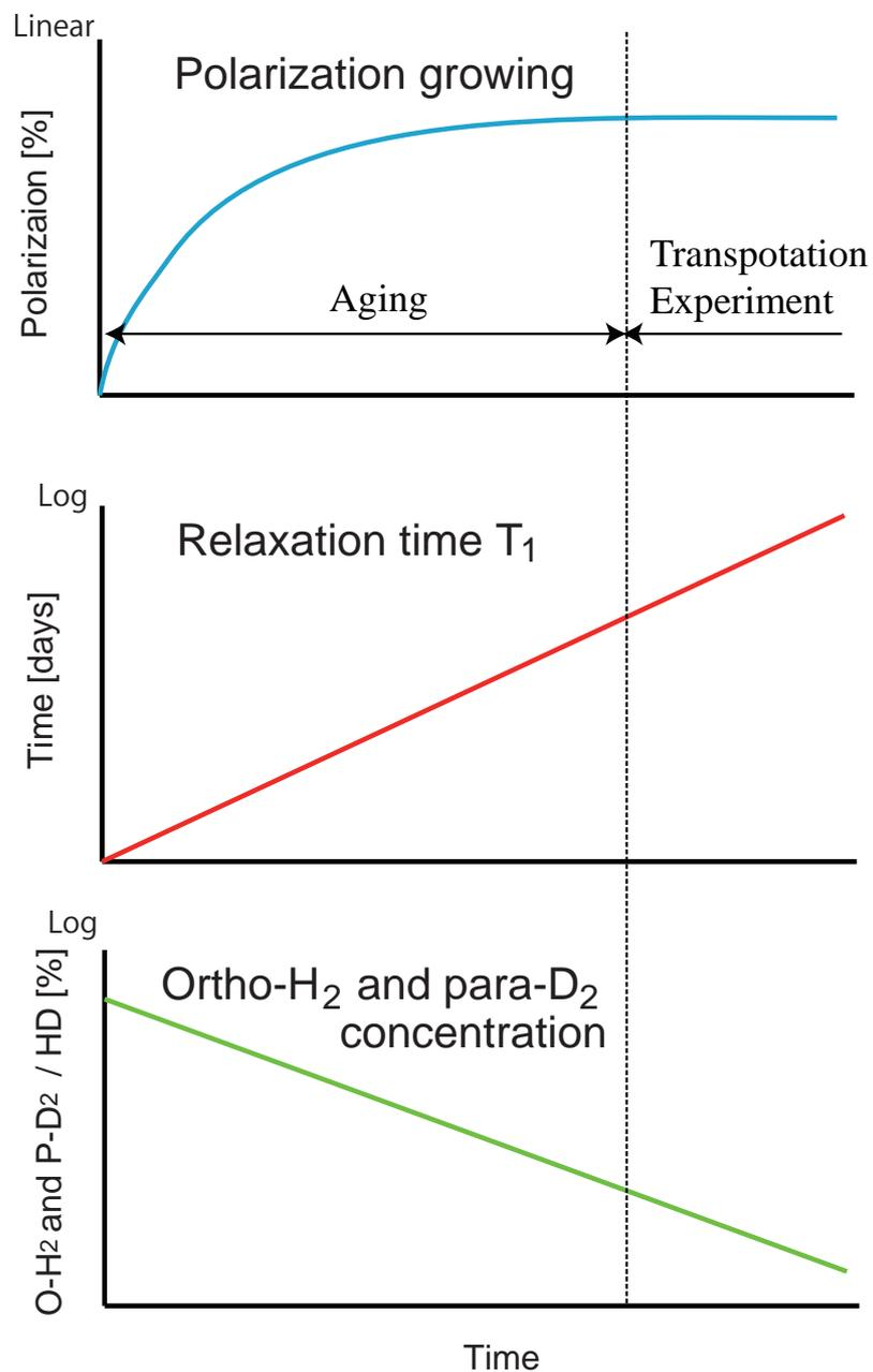
Figure 2.4: A model of frozen spin mechanism with elapsed day. The panels shows variances of the polarization, relaxation time and o-H<sub>2</sub> concentration in HD with elapsed day.
