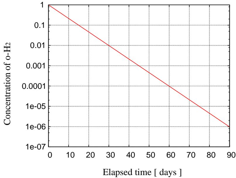
Figure A.1: Decaying the amounts of o-H<sub>2</sub> with elapsed days. The time constant of ortho-para conversion assumed to be 6.5 days.
