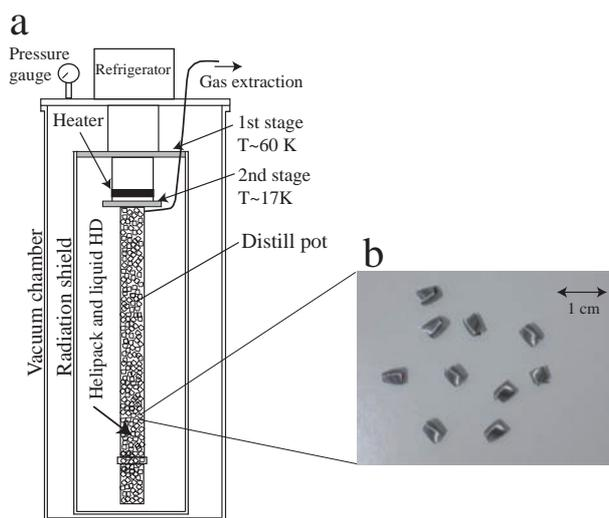
Figure 6.2: (a) The design view of the distillator. The  $H_2$  gas is extracted from the top of the distillation pot. (b) The photograph of stainless steel packs which are filled into the pot in the distillator. Each pack has a rolled shape like a coil and twisted for efficient heat conduction between gas and liquid.
