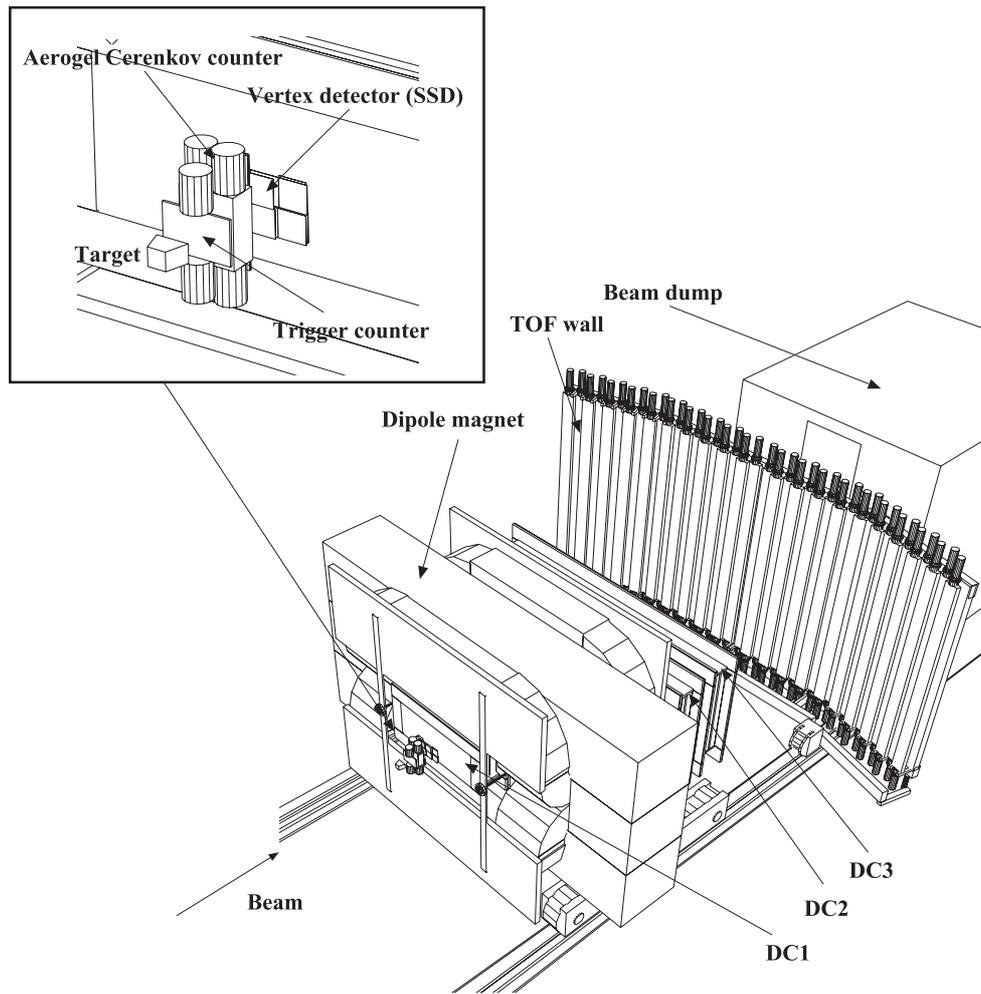
Figure 1.7: Top view of the LEPS detector in the experimental hutch. The photon beam is injected to the target from the left side. A typical event of  $K^+K^-$  pairs decaying from  $\phi$  meson is illustrated. Charged particles are bent by the 30 ton dipole magnet and their trajectories are determined by the multiwire drift chambers (DC's) triggered with the STC and TOF counters.
