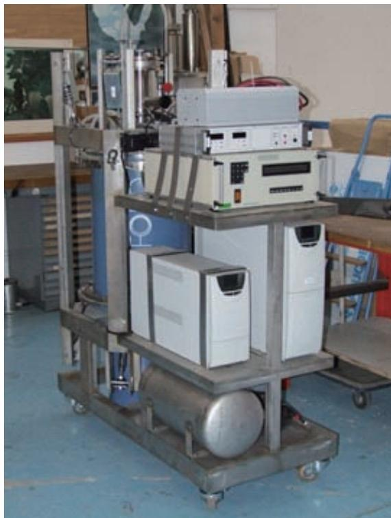
Figure 3.3: The photo picture of the Storage Cryostat (SC)
