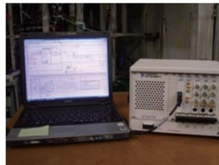
Figure 5.10: (a) The conventional NMR polarimeter system installed in a rack. Essentially, we need to prepare a signal generator, an oscilloscope, a lock-in amplifier, and a network analyzer. (b) The portable NMR polarimeter system consisting of a laptop PC and a PXI system.
