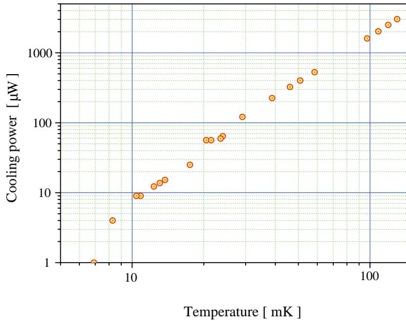
Figure 3.6: Measured cooling power of dilution refrigerator
