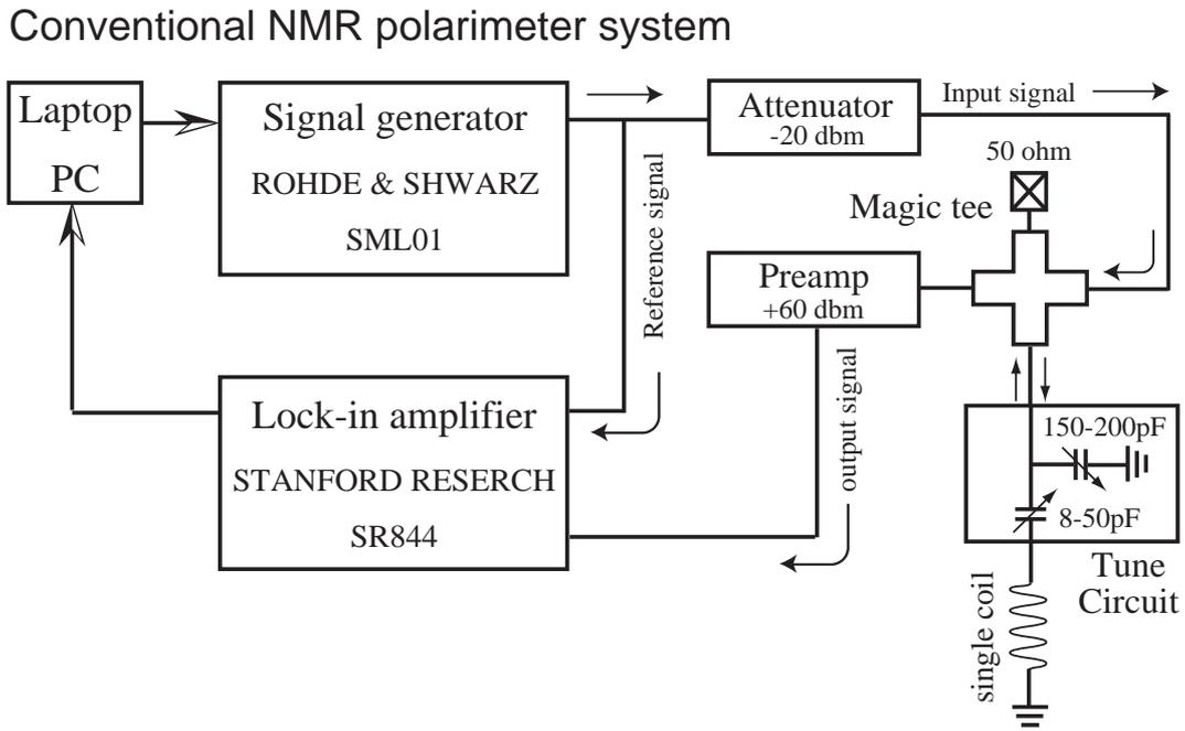
Figure 5.8: Schematic drawing of the conventional NMR polarimeter electronics.
