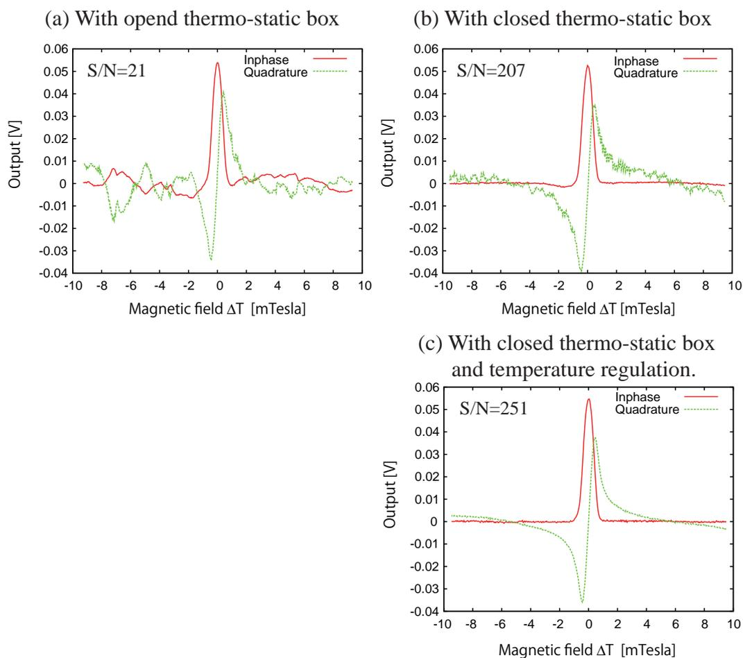
Figure 5.5: The measured NMR spectra with thermo-static box. (a) The NMR spectra with opened thermo-static box. (b) The NMR spectra with closed thermo-static box. (c) The NMR spectra with closed thermo-static box and temperature regulation.
