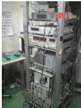
(b) Portable NMR polarimeter system
