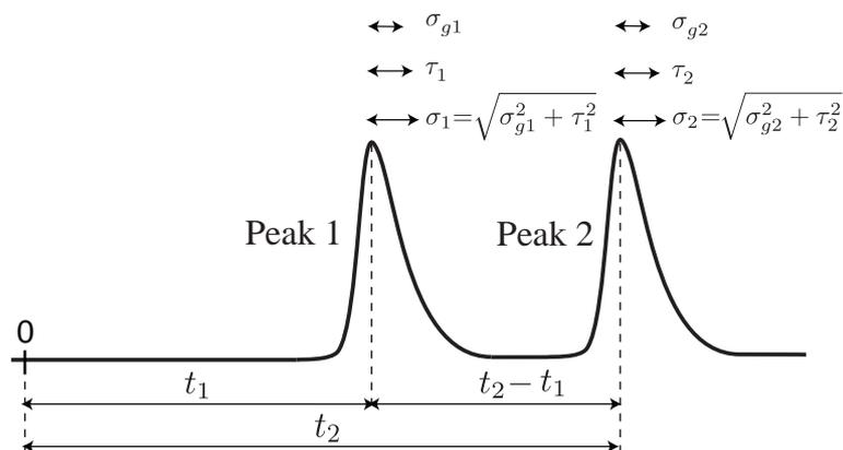
Figure 6.4: Expected peaks in the gas chromatography.  $t_1$  and  $t_2$  are the retention times.  $\tau_1$  and  $\tau_2$  are the time constant of the peak. The separation degree  $R$  is defined by Equation 6.2. Two peaks are separated completely with  $R > 1.5$ .
