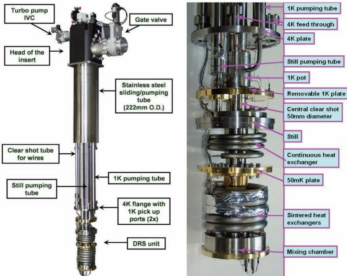
Figure 3.4: Photograph of the dilution refrigerator unit
