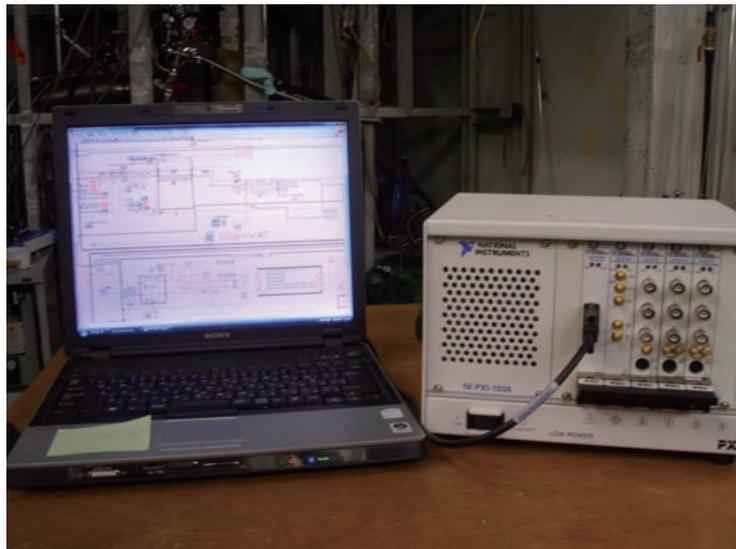
Portable NMR measurement system
