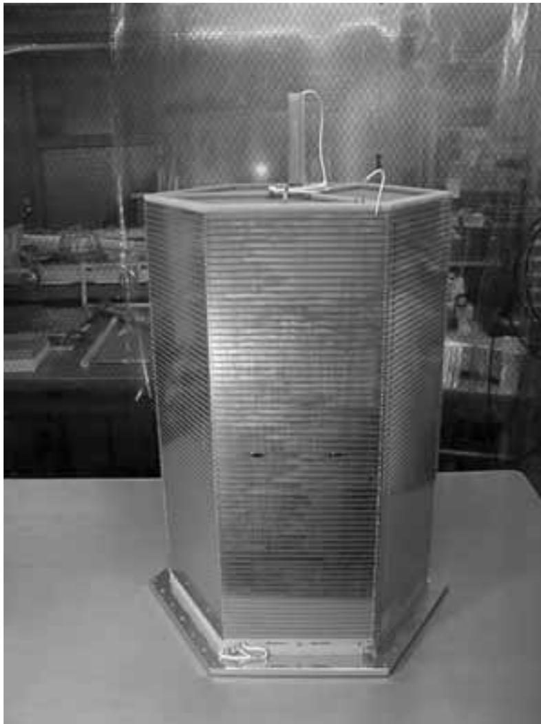
Figure 2.15: Picture of the field cage.
