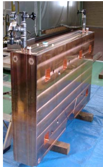
Beam dump core after waterway drilling
