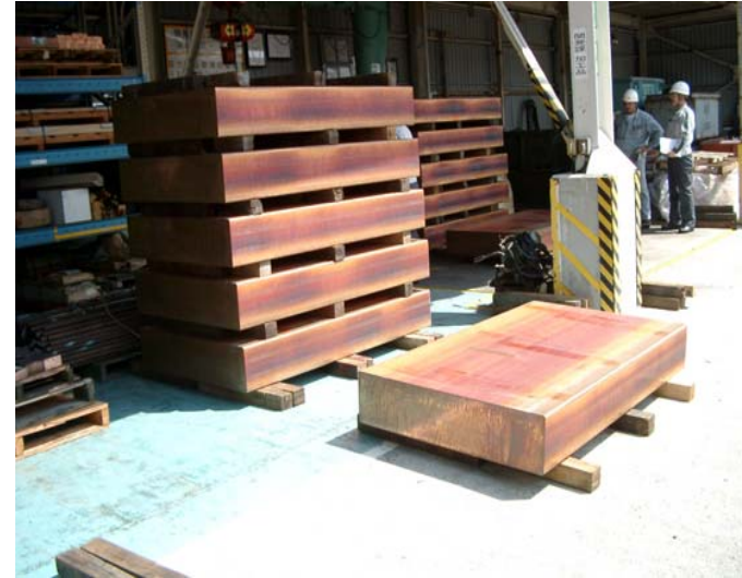
Beam dump core made of OFC
