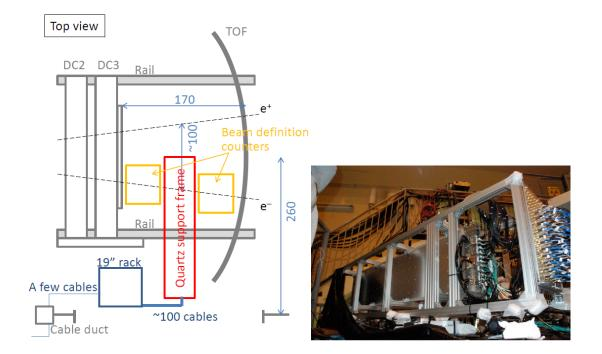
We have produced a prototype TOP counter (see picture) to check the demonstrated overall timing performance. The prototype consists of 1830 x 400 x 20 mm<sup>3</sup> quartz radiator with a spherical focusing mirror (5m radius) and the 14 MCP-PMT array. The signal from MCP-PMT will be read out by compact CFD electronics and TDC.
