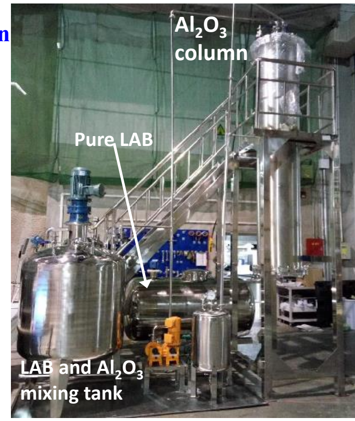
Al 2 O 3 column pilot plant installed in Daya Bay LS hall
