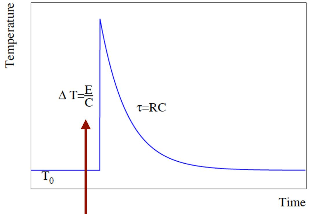
Energy Deposition causes rise in temperature inversely proportional to the heat capacity.
