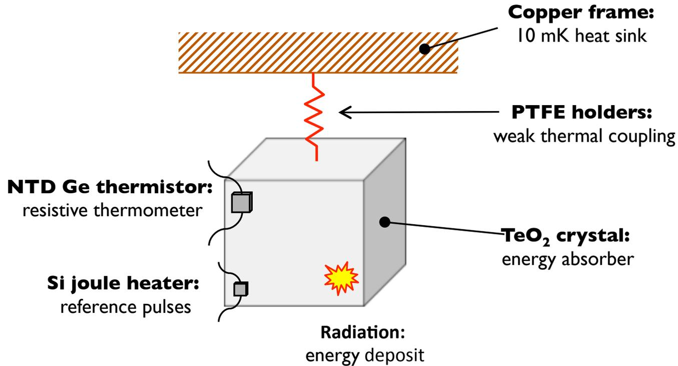
**Heat Measurement: Absorber + Thermometer**
