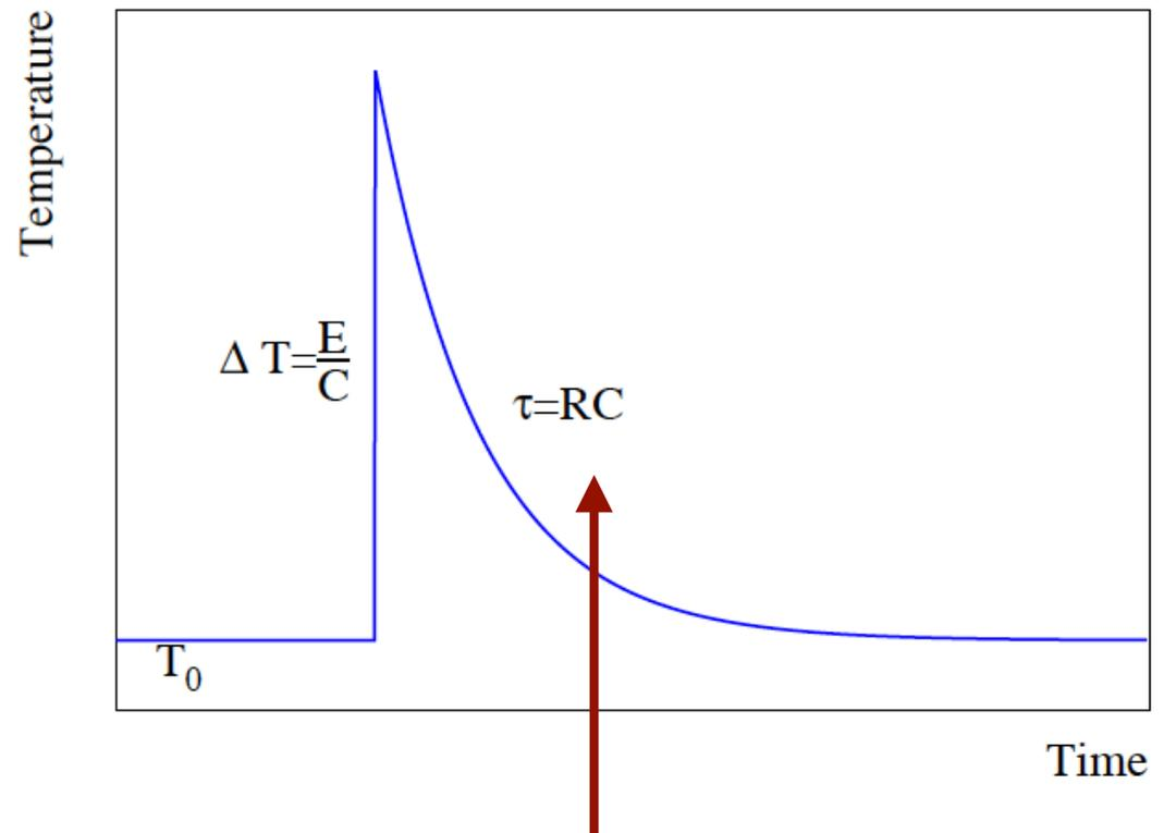
The decay time of the signal is proportional to the thermal resistance.
