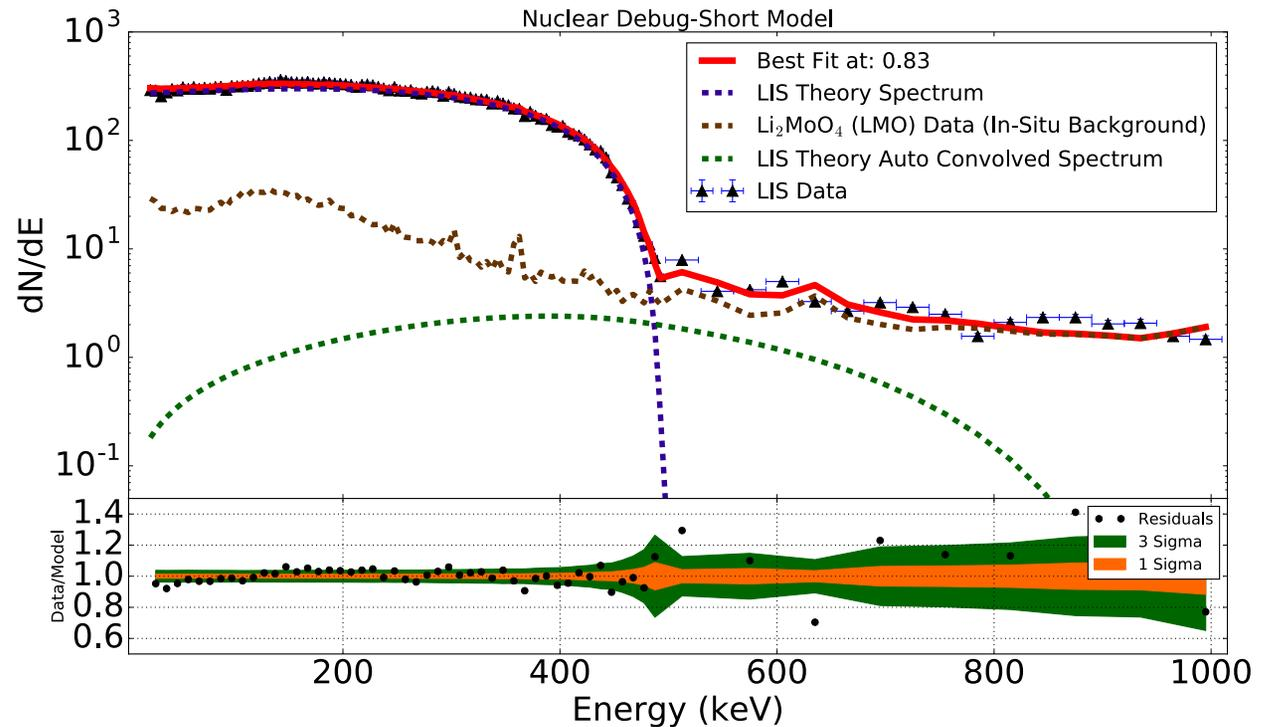
*The highly forbidden  $^{115}\text{In}$  decay prevents this crystal from being viable for CUPID, but the precision spectrum measurement can inform the nuclear matrix calculations (quenching of  $g_A$ ).*
