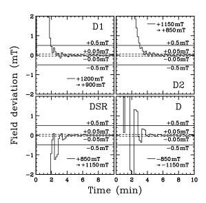
Figure 2: Typical magnetic field responses of the dipole magnets D1, D2, and DSR of Grand Raiden, and the magnet D1 of Large Acceptance Spectrometer.
