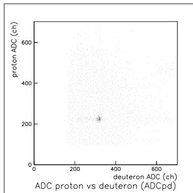
Figure 3: Two dimensional plot of the light output of the deuteron and the proton counters.
