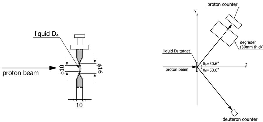
Figure 1: Side view of the target cell for the SND search experiment.
