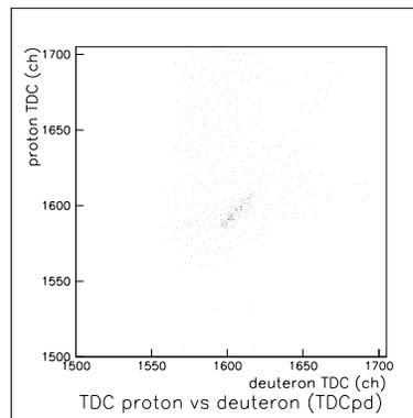
Figure 4: The plot of timing information of the deuteron and the proton counters.
