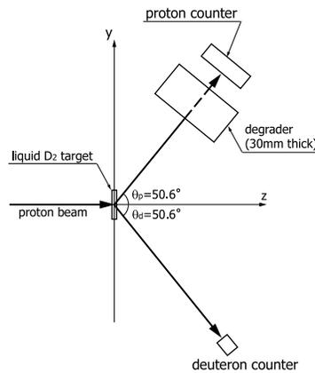
Figure 2: Schematic view of the luminosity monitor. The plastic scintillation counters are placed at 20 cm downstream of the target.
