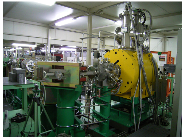
Figure 3. 18 GHz ECR ion source and beam line.
