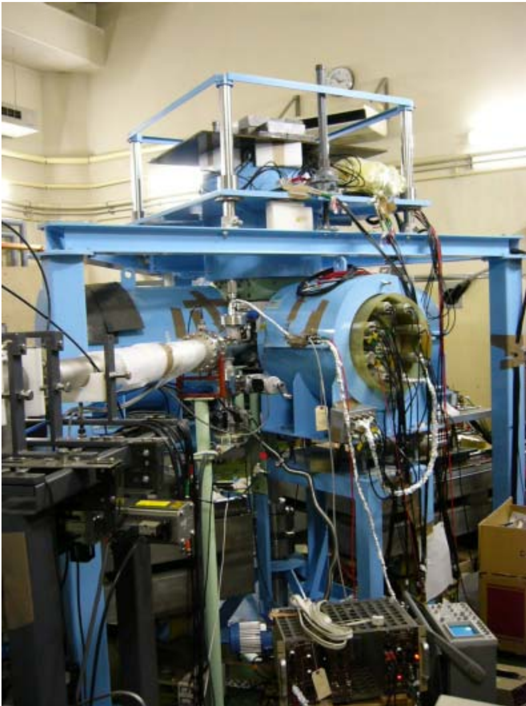
Figure 1: Photograph of the \gamma -ray detector system for measurement of the ^{12}\text{C}(\alpha, \gamma)^{16}\text{O} reaction cross section.
