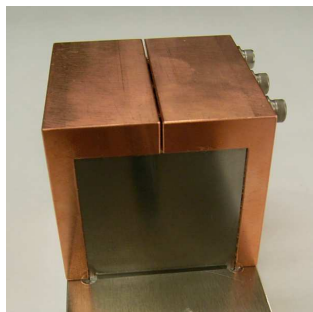
Figure 1: Tungsten target for the white neutron production.
