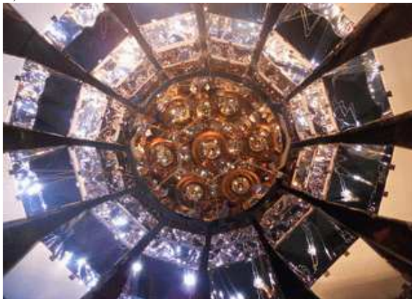
Figure 2: a) Inside view of the water tank. The light-concentration system, which has mirror-reflector films, are installed in front of the photomultiplier tubes. b) Result of the position reconstruction analysis. The peaks of the reconstructed position have 6\sigma separation for each \text{CaF}_2 (pure) scintillator.
