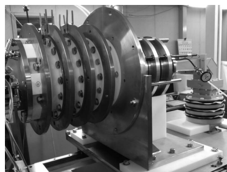
Figure 2: A 2.45 GHz proton source.
