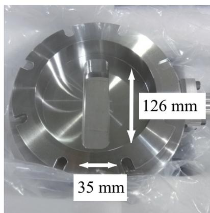
Figure 2: Fast closing shutter.
