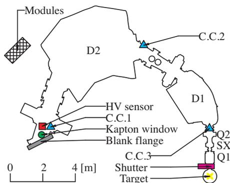
Figure 1: Schematic view of the GR and the layout of the fast closing system. The layout of the examination is also shown.
