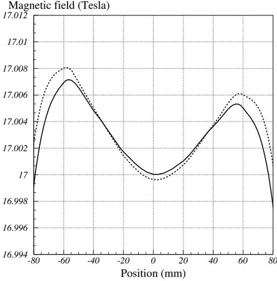
Figure 2: Magnetic field around the center of the super-conducting magnet. The solid and dashed curves are at  $R=0$  cm and  $R=1.5$  cm, respectively.
