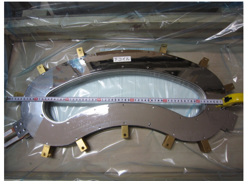
9mm and 4.5mm thick iron plates were put on outside and inside of a coil, respectively.
