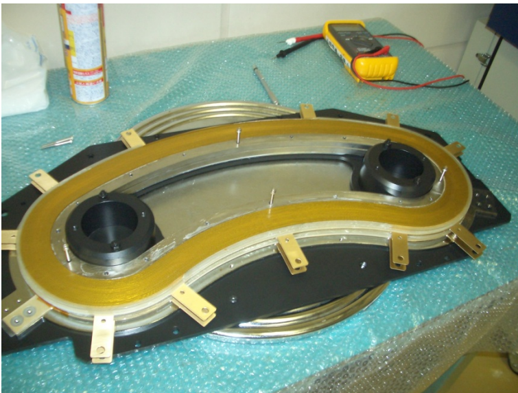
Three DP and cooling plates are stacked and fixed with epoxy resin in vacuum.
