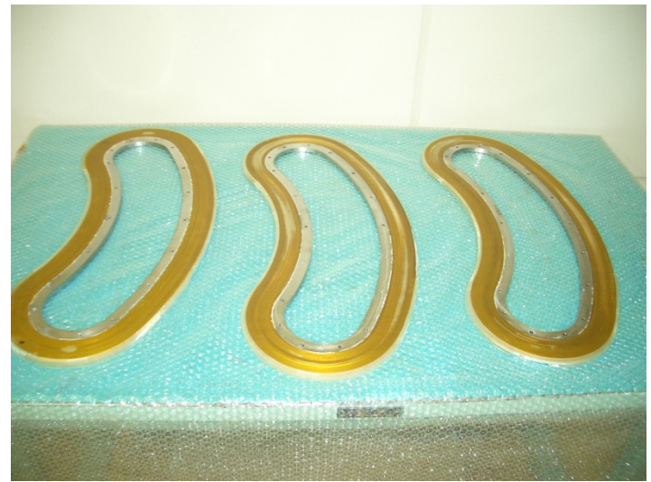
Each DP was fixed with epoxy resin in vacuum.
