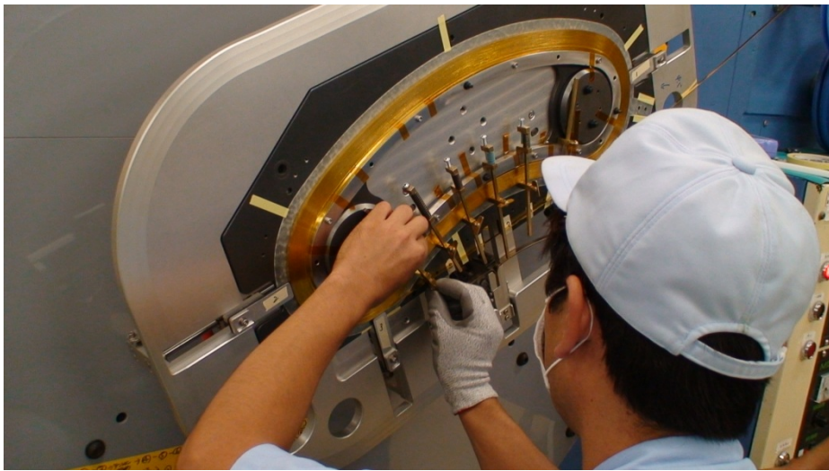
Double pancake (DP) was wound with applying tensile stress.
