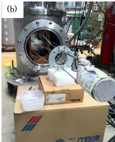
Fig. 9: (a) Drawings of the deuteron target system (side view). A double-stage G-M refrigerator is used to liquefy the deuterium at the heat exchanger. Liquid deuterium is filled in the target cell through a long transfer tube. (b) A photograph of the target cell connected with the heat exchanger via transfer tubes. The cell is surrounded by super insulator films as a radiative heat load protection. (c) A photograph of the target system.
