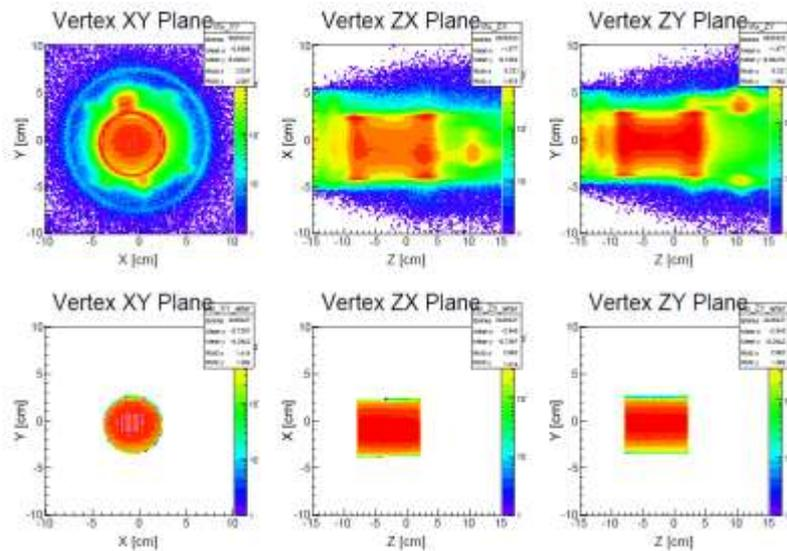
Fig. 3: Reaction vertex determined from a beam track and a charged track in CDC by means of the closest distance approach. An image of the target cell was clearly observed (upper). The target deuterium was selected by a fiducial volume cut (lower).
