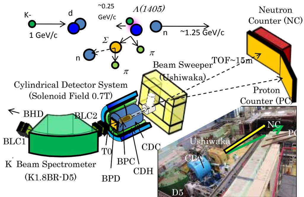
Fig. 1: Layout of the experimental setup for the E15/31 experiment
