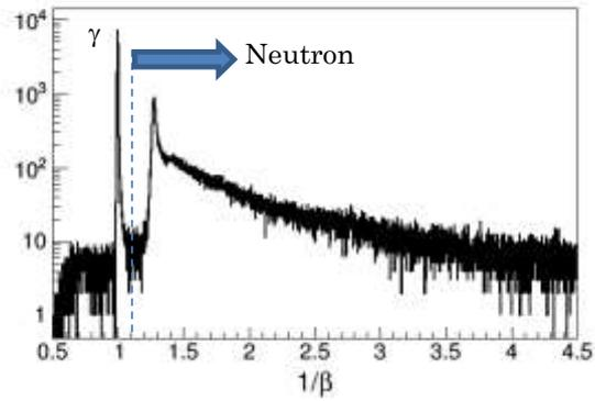
Fig. 4:  $1/\beta$  spectrum obtained by the neutron time of flight counter located at a distance of 15 m from the target. A peak of gamma rays is located at  $1/\beta=1$ . Neutrons are identified in the region of  $1/\beta > 1.1$ .
