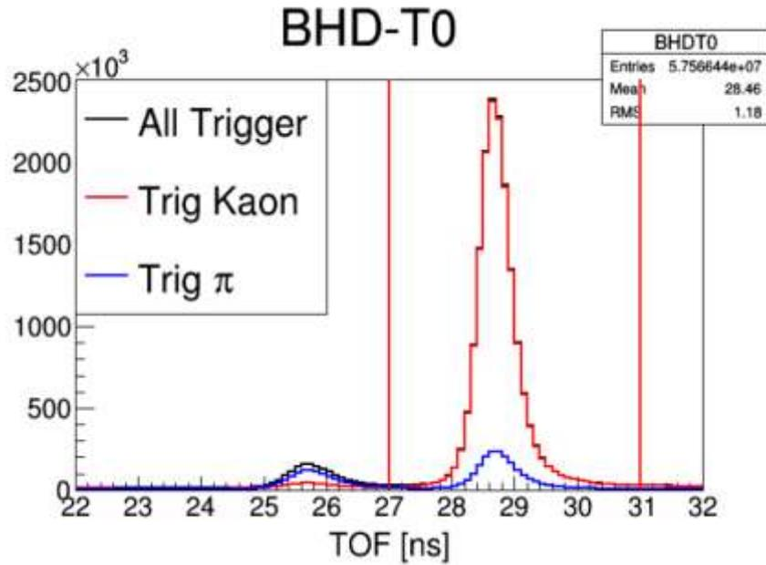
Fig. 2: Time of flight between BHD and T0 counters. BHD is beam hodoscopes located at the most upstream in the beam line of the K1.8BR experimental area. T0 is a time zero counter hodoscopes located upstream of the target. Vertical red lines indicate a time window for selecting kaon beam.
