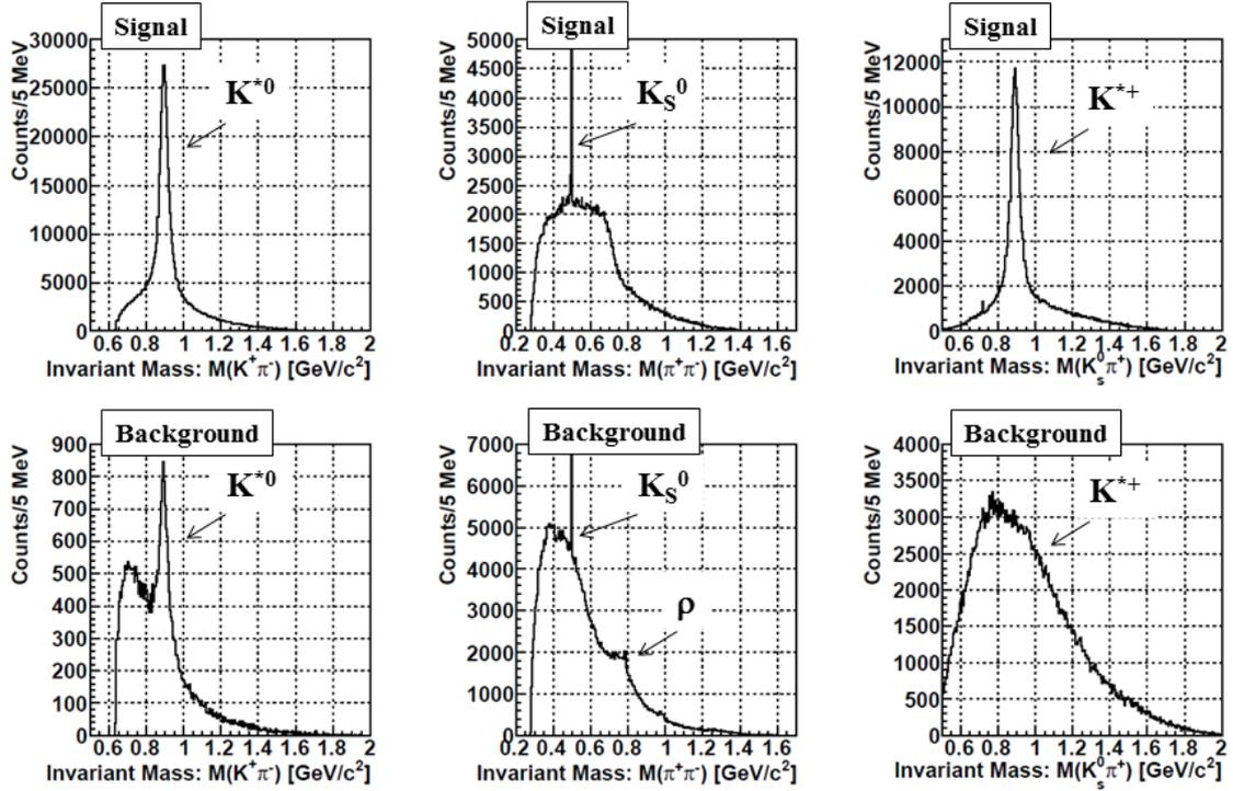
FIG. 3: Reconstructed  $K^{*0}$  (left),  $K_s$  (middle), and  $K^{*+}$  (right). Top figures show only for signals, and bottom ones only for background events generated by JAM.
