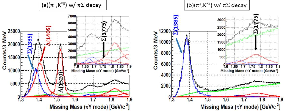
FIG. 9: Simulated missing mass spectra of the  $p(\pi^-, K^{*0})$  (left) and  $p(\pi^+, K^{*+})$  (right) reactions with gating the  $\pi^+\Sigma^-$ -decay mode are shown including the  $\Lambda(1405)$  resonance region.
