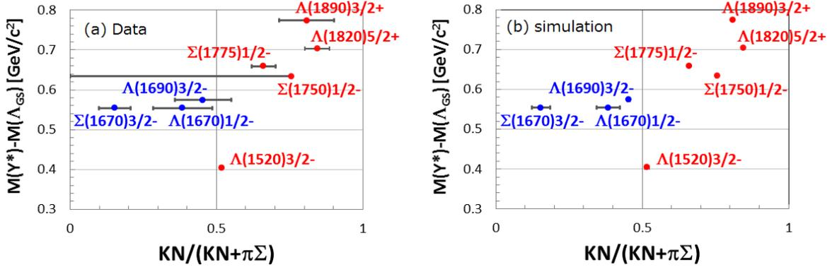
FIG. 8: The ratios of the hyperon decay rate to  $\bar{K}N$  with the sum of the decay rates to  $\bar{K}N$  and  $\pi Y$ . Phase space corrections are made with assuming an allowed lowest wave in a decay. (left) The ratios are plotted based on the PDG data [7]. (right) Expected improvement of the ratios estimated by simulations. The errors are expected at a level of a few %.
