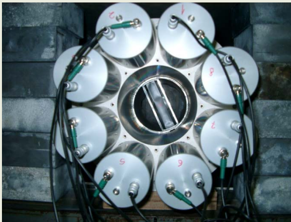
The 8.54 l BGO 16-section scintillation detector: NIM A517 (2004) 269 Used for ^{237}\text{Np}(n, \gamma) : JNST 42 (2005) 135
