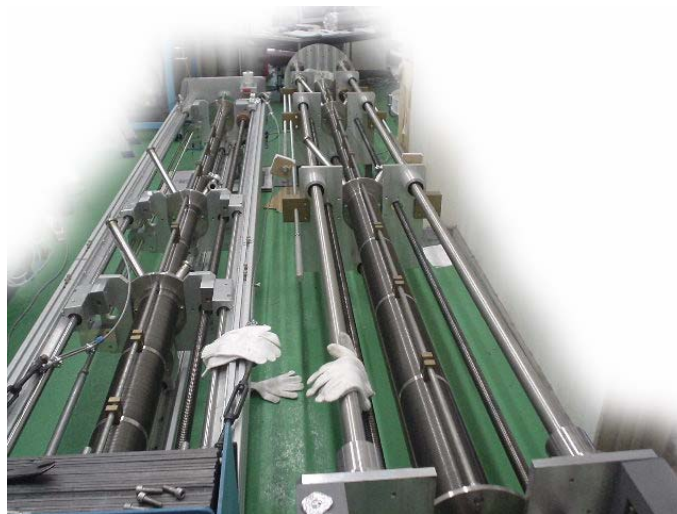
Figure 2.9: The left side of the figure is TC1, which is mainly for moving the target from the DRS to the SC. The right side the figure is TC2, which is mainly for moving the target from the SC to the IBC.
