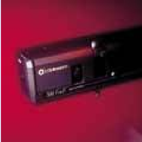
Coherent : Innova Savre MOTOFRED Ar-laser + BBO CW 1W, \lambda=257.2 nm Power consumption 10 kW
