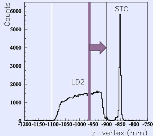
Proton rejection efficiency becomes **60%→90%** by selecting downstream of target
