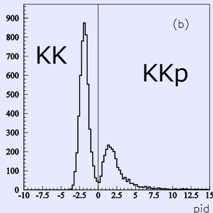
Proton detection by using  $dE/dx$  in the start counter
