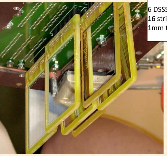
6 DSSSD detectors 1mm with 16 strips X and 16 strips Y, 1mm thick, 5 x 5 cm area
