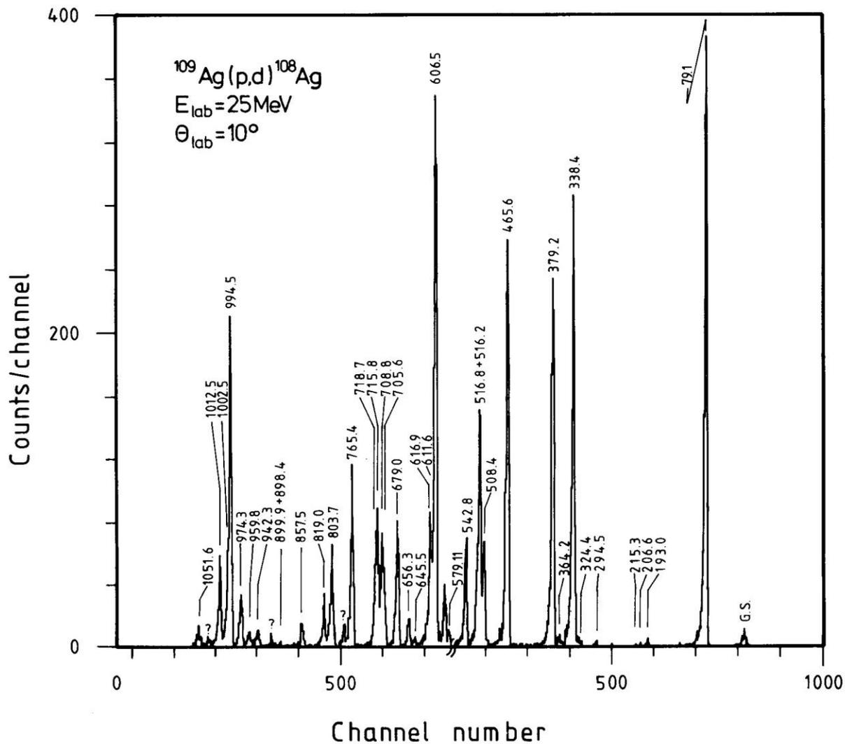
Fig. 19. High resolution spectrum of the  $(p,d)$  neutron pick up reaction on  $^{109}\text{Ag}$  at 25 MeV incident energy and a solid angle of 1.2 msr. The resolution was 4 keV.
