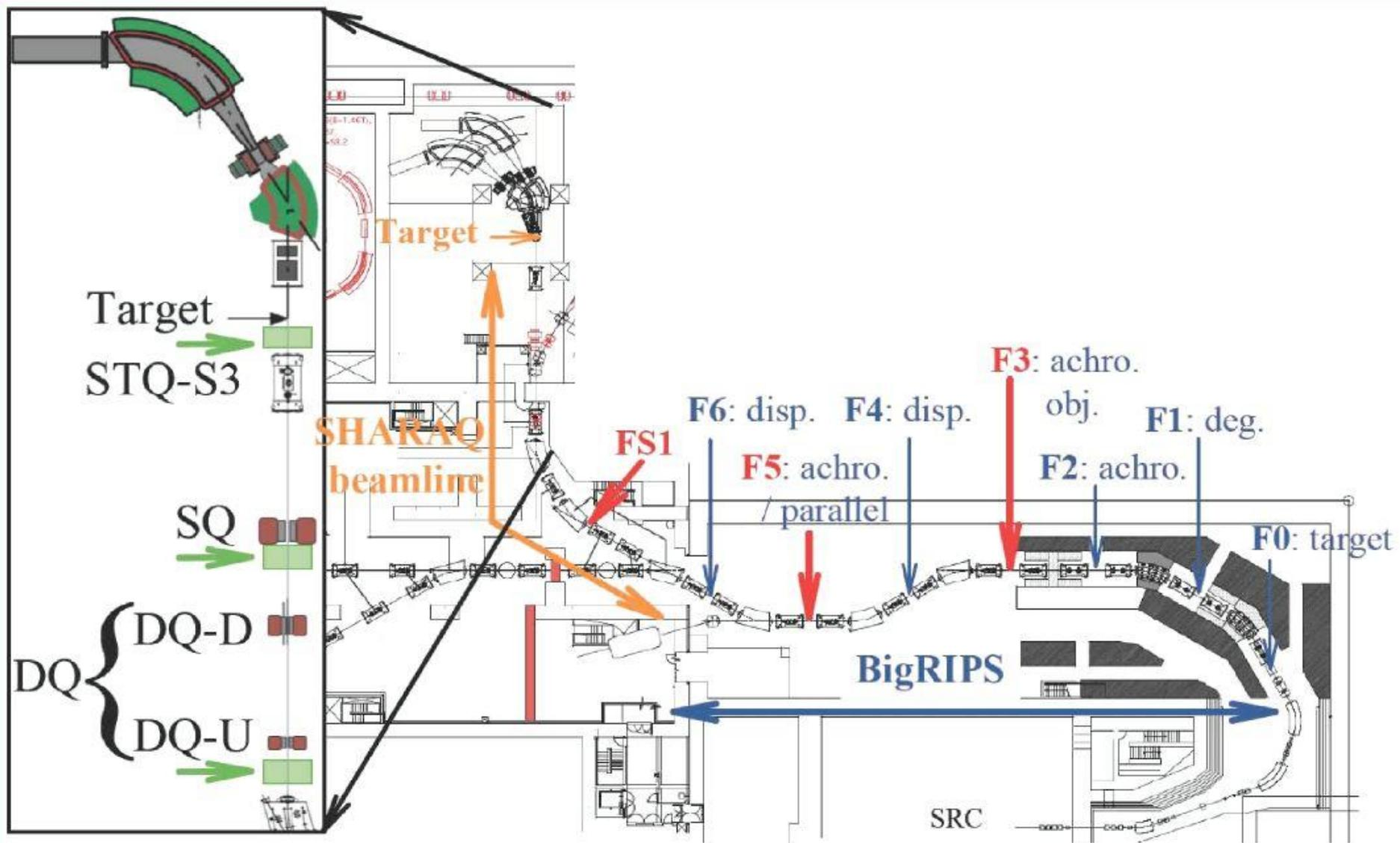
**FIGURE 3.** Dispersion-matched beam-line for the SHARAQ spectrometer. The RI beams produced at F0 are transported to the SHARAQ target through the BigRIPS beam-line and the SHARAQ beam-line. The dispersive beam transport starts from the achromatic focus at F3.
