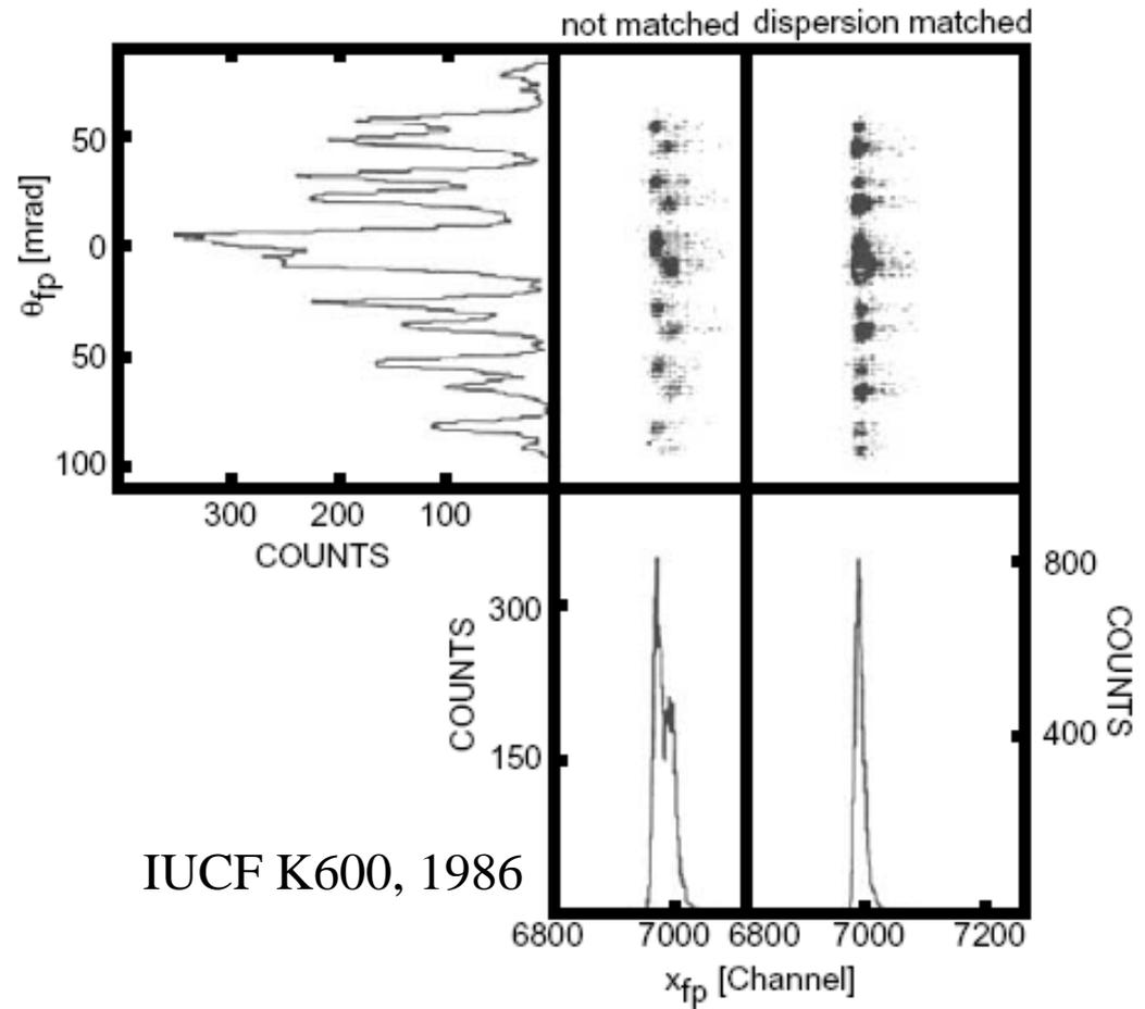
Fig. 4. Scatterplots of horizontal position  $x_{fp}$  versus angle  $\theta_{fp}$  and projections measured in the focal plane of the K600 using the "multi-slit system". For details, see text.
