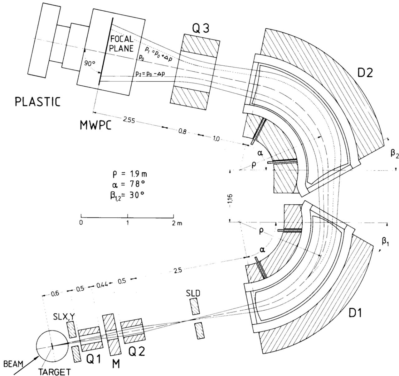
Fig. 9. Arrangement of the magnetic elements of the QDQDQ spectrometer BIG KARL. The central ray (optical axis) is shown as dashed curve. The outermost rays with the extreme radial distances are drawn as full lines. Four channels in the inner yokes allow NMR probes to be moved into the gaps of the dipoles for radial field measurements. The multipole element between Q1 and Q2 allows the correlation of vertical aberration.
