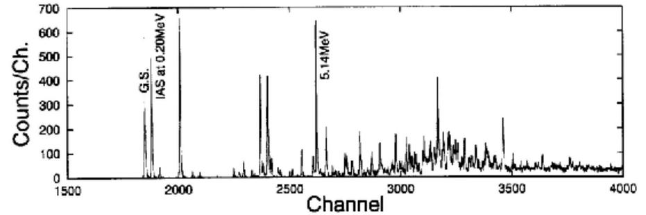
Figure 4.4: Spectrum of  $^{58}\text{Ni}(^3\text{He},t)$  reaction. The lateral and angular dispersion matching technique and over-focus mode were applied in this experiment for high energy and scattering angle resolution. Energy resolution of about 30 keV (FWHM) was realized.
