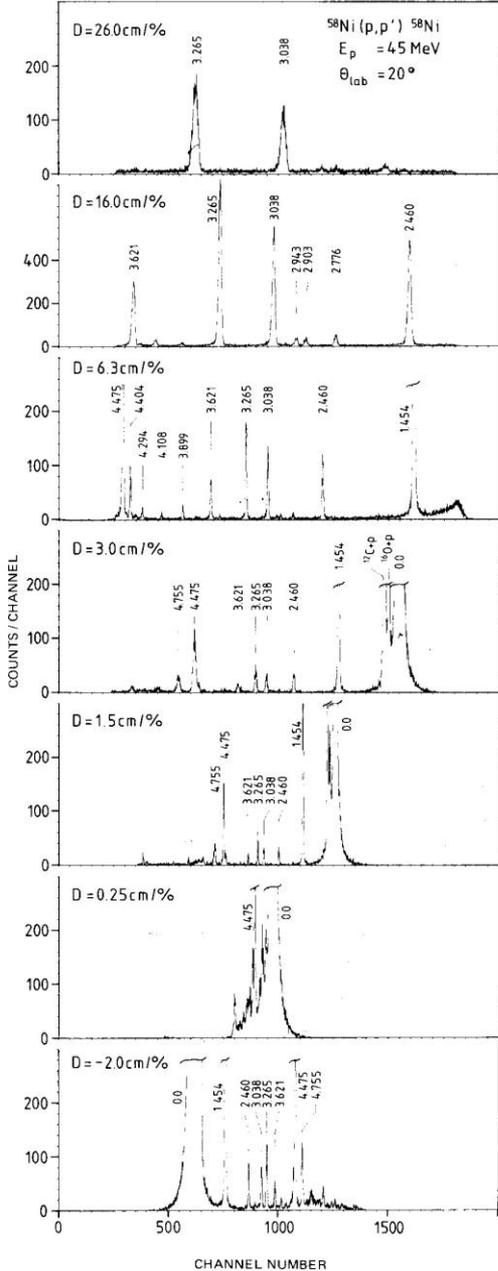
Fig. 4. Spectra of  $^{58}\text{Ni}(p,p')$  measured for different dispersions  $D = 26, 16, 6.3, 3, 1.5, -0.25$  and  $-2\text{ cm}/\%$ . The spectrograph was optimized for  $D = 16\text{ cm}/\%$ .
