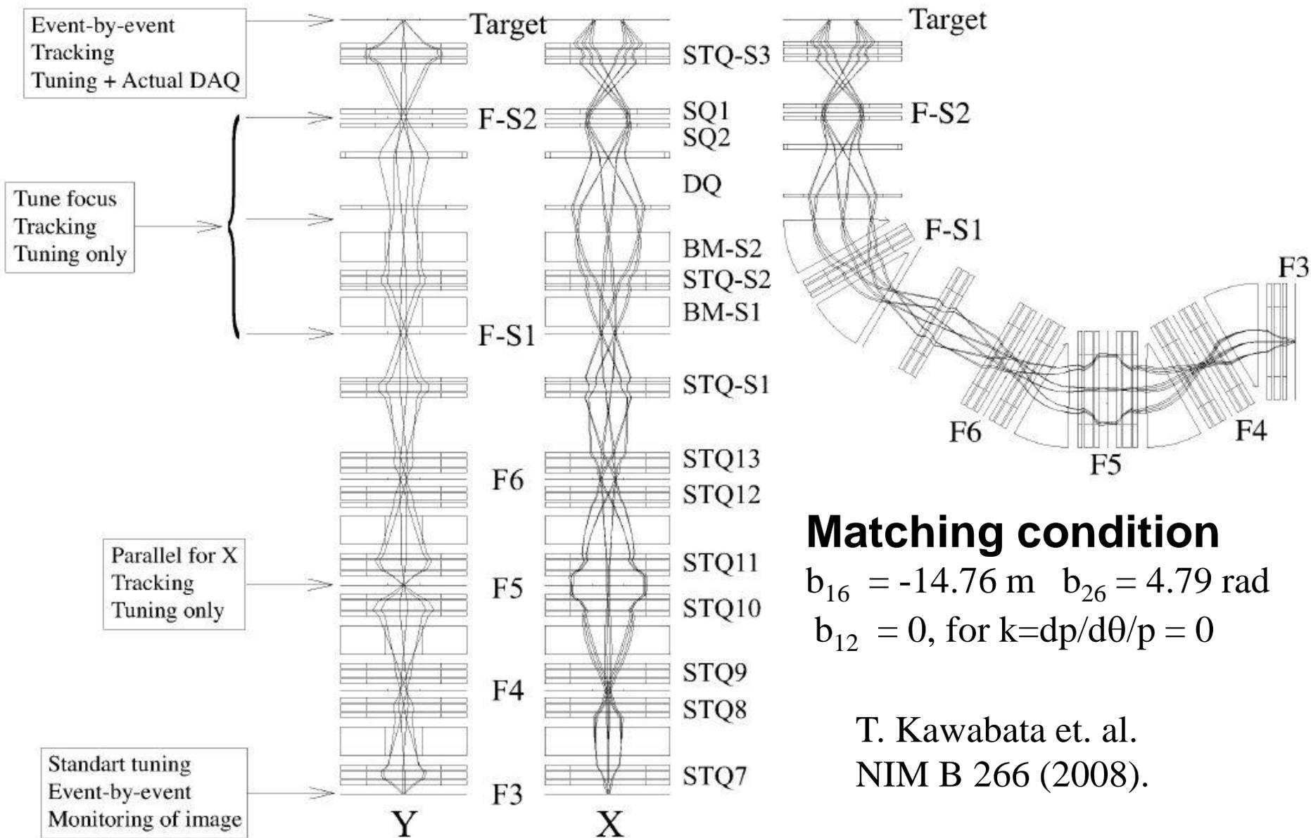
**FIGURE 4.** Calculated optics of the dispersive beam transport from F3 to the SHARAQ target.
