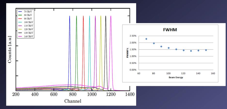
Spectra of protons at different beam energies measured with a 2" x 2" x 2" LaBr<sub>3</sub>:Ce crystal at 5 deg. relatively to the beam axis. The spectra are normalized to have the same height of a proton peak.
