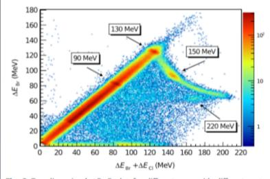
**Fig. 6.** Two-dimensional  $\Delta E - E$  plot for different runs with different proton energies: 90, 130, 150 and 220 MeV. The vertical axis represents the energy deposited in the LaBr<sub>3</sub> crystal and the horizontal axis the total energy deposited in the phoswich.
