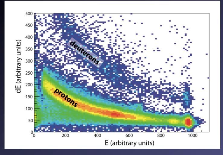
BINA particle identification spectrum
