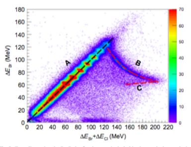
**Fig. 8.** Two-dimensional  $\Delta E - E$  plot for the runs included in the resolution analysis (protons of 70–230 MeV). The 2D histogram has been later projected onto the three lines: A, B and C for the determination of the energy resolution (see the text).
