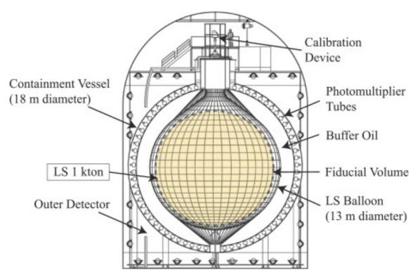
Fig. 1.5 Schematic view of KamLAND detector.
