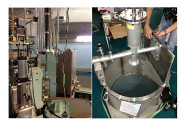
Fig. 2.2 Target ladder system (left) and scattering chamber (right).
