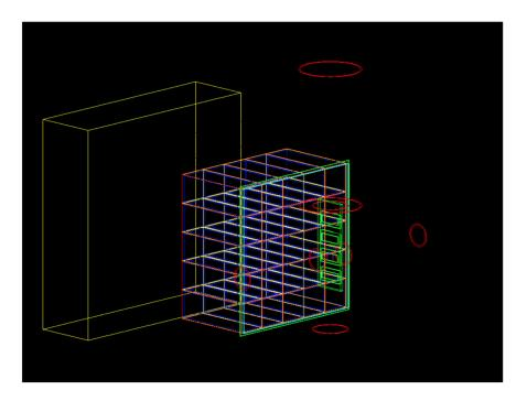
Fig. 3.3 Geometrical set up in the MC simulation depicting various components and materials (Blue = NaI).
