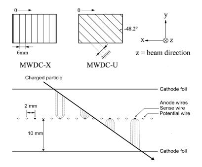
Fig. 2.5 Wire configuration (up) and structure (down) of MWDC [1].
