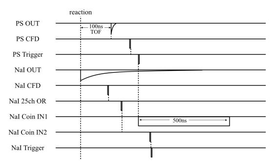
Fig. 2.14 Timing chart of signals.
