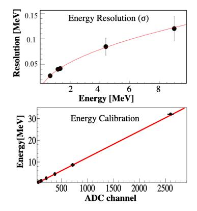
Fig. 2.8 Energy resolution and pulse height response of a NaI counter.
