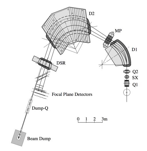
Fig. 2.3 Magnetic spectrometer "Grand Raiden" [1].
