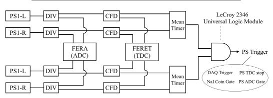
Fig. 2.12 Circuit diagram of the plastic scintillators.
