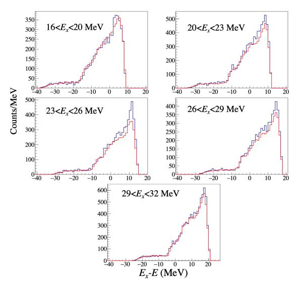
Fig. 3.11  $E_x - E$  spectra (blue) for different  $E_x$  regions with background spectra (red line).
