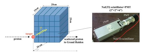
Fig. 2.6 An array of  $\gamma$ -ray detector (left) and a NaI(Tl) scintillation counter (right).
