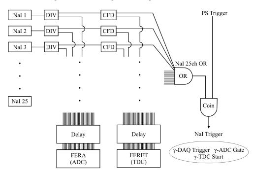
Fig. 2.13 Circuit diagram of PS Trigger and NaI Trigger.
