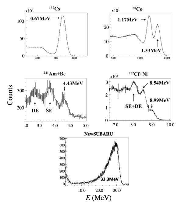
Fig. 2.7 The energy spectra taken by radioactive sources. SE (DE) denotes single (double) escape peak.
