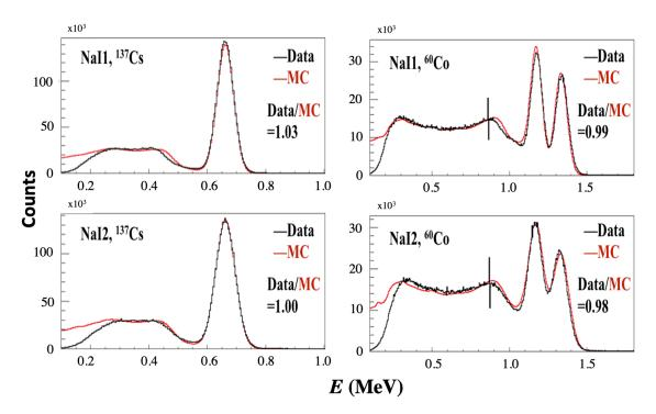
Fig. 2.9 The measured energy spectra (black) and normalized response function (red). Data/MC shown in the figures is the number of events from the data divided by that from the normalized response function with energy higher than 0.3 MeV for <sup>137</sup>Cs and 0.5 MeV for <sup>60</sup>Co.
