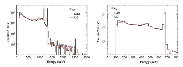
Fig. 6.1 Energy spectra observed by peripheral crystal 6 of the upper cluster in our data (black) and our MC (red) for the calibration sources  ${}^{60}$ Co (left) and  ${}^{137}$ Cs (right).
