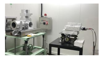
Fig. 2.11 NaI(Tl) detector (same used for E398 experiment) used for measuring 33 MeV  $\gamma$ -rays at NewSUBARU facility.
