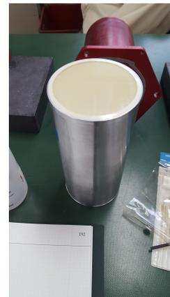
Figure 2.9: Large volume  $\text{LaBr}_3$  detector and the crystal [GIA13].
