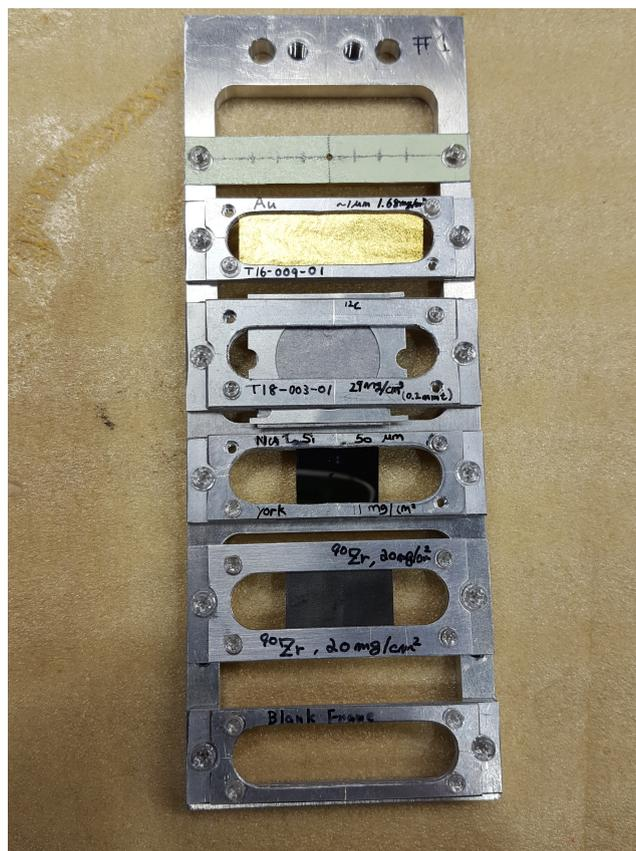
Figure 2.16: Target ladder with targets and a viewer.
