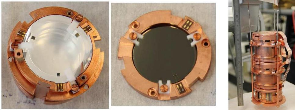
Main crystal, Ge wafer cryogenic light detector readout by NTDs
