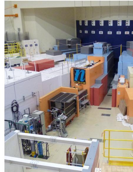
Spallation neutron target (designed for 1MW)
