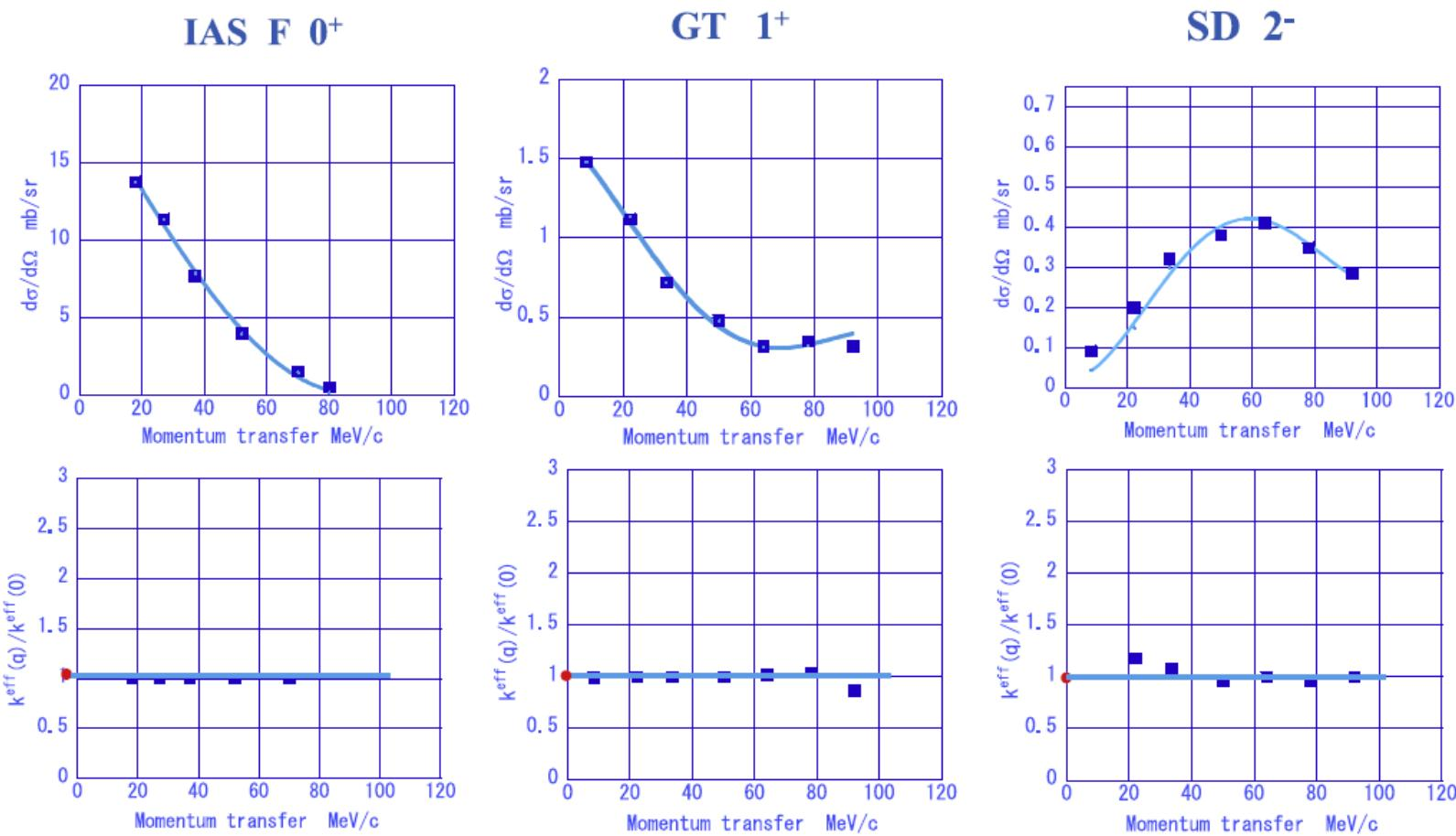
Fig. 15. Top: The  $^{76}\text{Ge}(^3\text{He},t)$  CER cross sections as functions of the momentum transfer  $q$  [95]. F  $0^+$ ; 8.31 MeV IAS, GT  $1^+$ ; the 0.12 MeV GT state, SD  $2^-$ ; the ground SD state. The solid lines are the DWBA calculations. Bottom: The ratio  $k_{\text{eff}}(q)/k_{\text{eff}}(q = 0)$  for  $\alpha = \text{F}$  (IAS), GT (1st GT state), and SD (ground state). The red point is the normalization point at  $q = 0$ . See [103].
