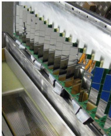
To wall of **2500 SiC-SiC-SiC** pad **telescopes**
