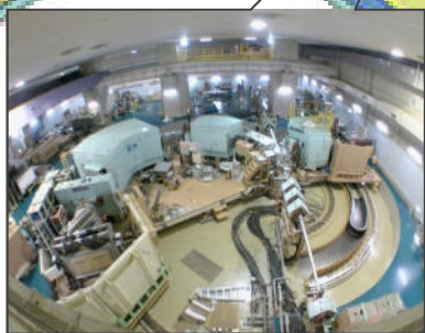
Double arm spectrometer (Grand Raiden & LAS)
