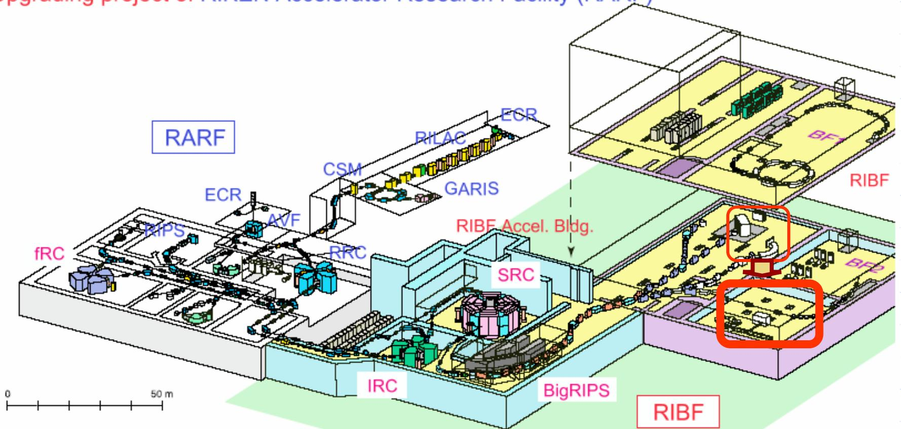
RIBF RI beam generator featuring superconducting ring cyclotron (SRC) and projectile fragment separator (BigRIPS) will be commissioned late in 2006.
