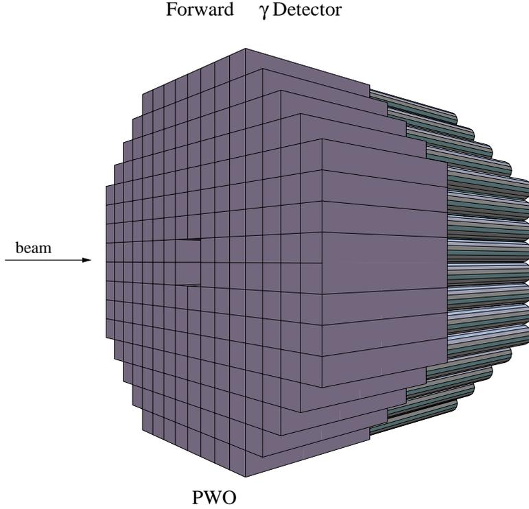
Figure 2: Drawing of the forward  $\gamma$ -detector system consisting of 252 PWO crystal scintillators.
