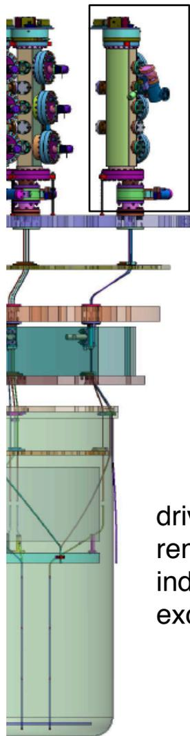
drive spools can be removed for individual source exchange
