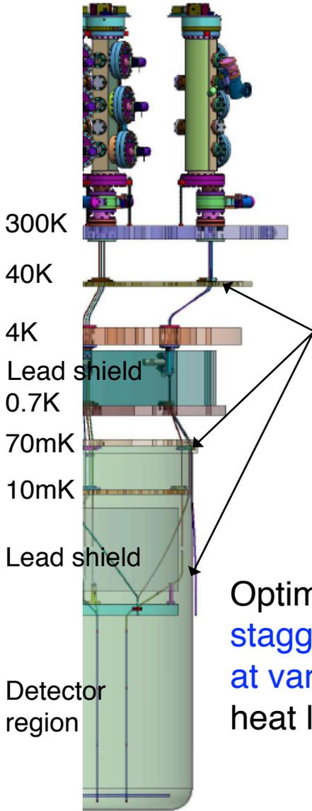
Optimize sequence of staggered source extraction at variable speed to meet heat load requirements
