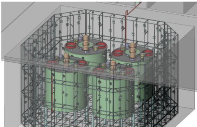
Inner and outer veto separated by Tyvek panels
