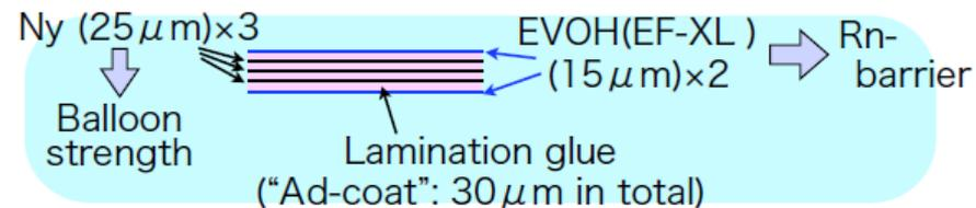
Film connection is made by sandwiching an EVOH film (no-extended type) and heat welding with microwave.
