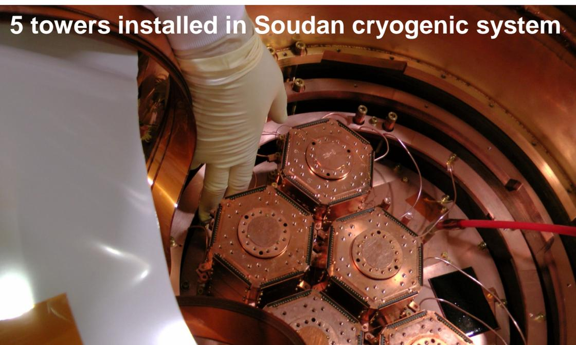
5 towers installed in Soudan cryogenic system
