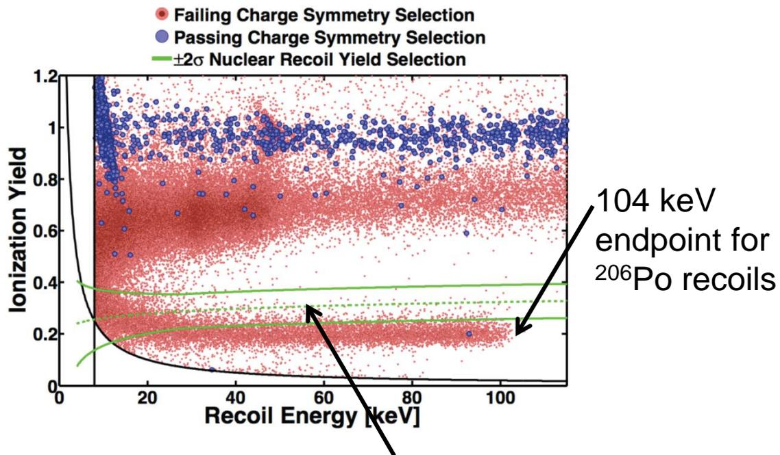
No symmetric (blue) events in nuclear recoil band for exposure equivalent to full SuperCDMS SNOLAB expt
