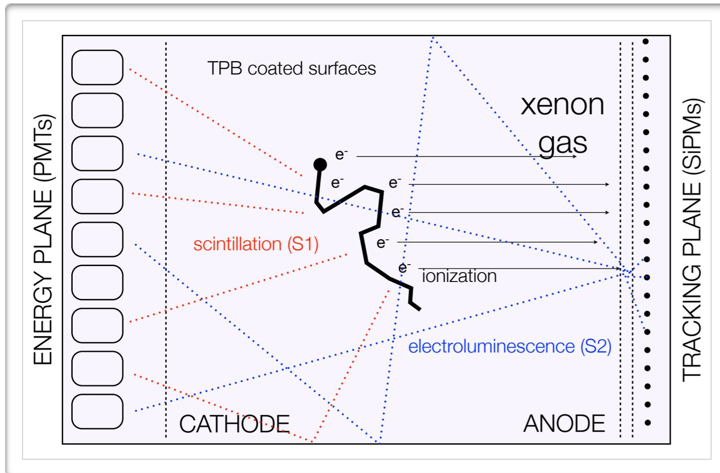
EL mode is essential for linear gain, avoiding avalanche fluctuations and fully exploiting the excellent Fano factor in gas
