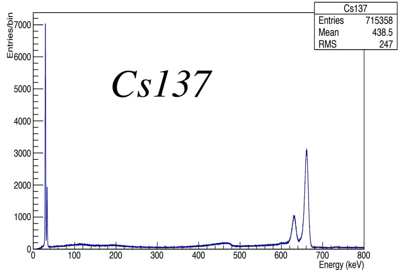
Reconstruction of events from  $^{22}\text{Na}$  and  $^{137}\text{Cs}$  result in energy resolutions of 1.62% and 1.58%. These values predict an energy resolution at  $Q_{\text{BB}}$  of  $\sim 0.75\%$  FWHM.
