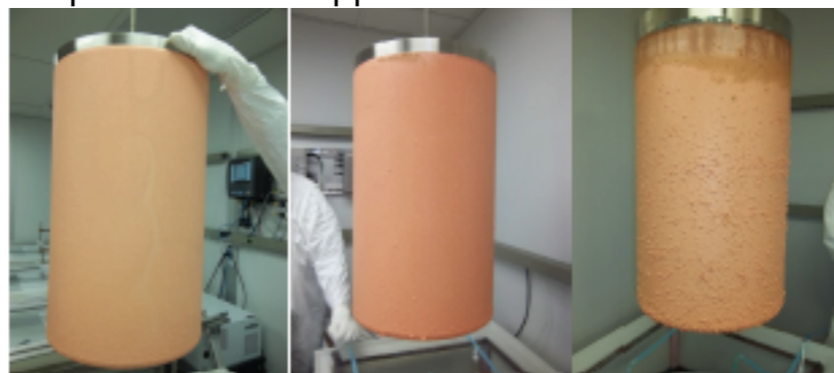
Inspection of EF copper on mandrels
