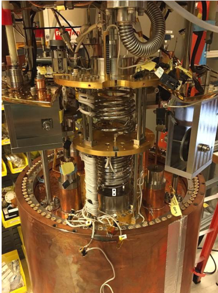
Dilution Refrigerator installed above ADMX Cavity
