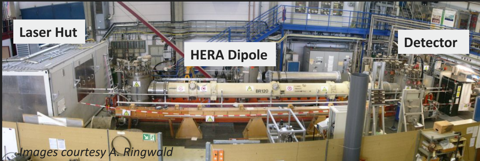
Implemented with lasers, dipole magnets. Resonant enhancement possible
