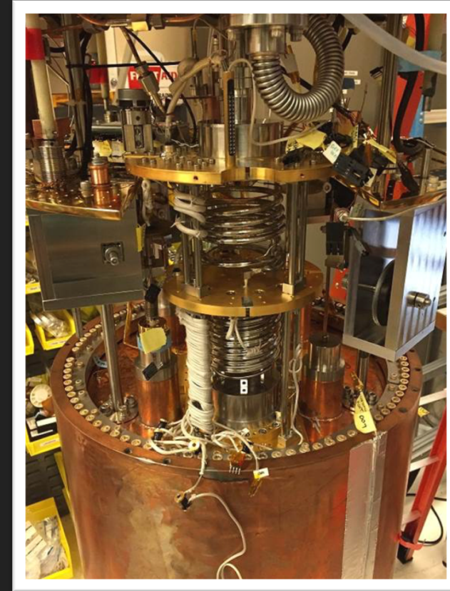
Dilution refrigerator installed above cavity
