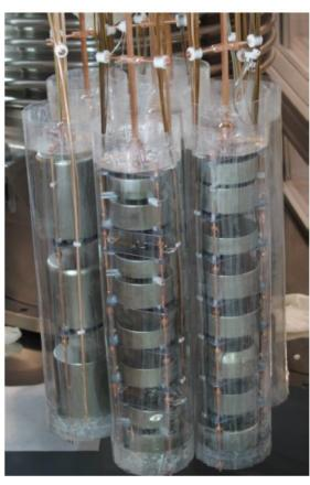
New TPB coated nylon minishrouds to reduce attraction of <sup>42</sup>K ions (from decays of <sup>42</sup>Ar) to n<sup>+</sup> surface
