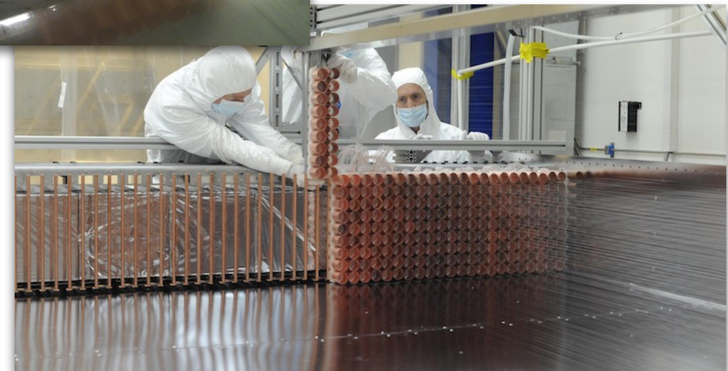
**2034** drift cells (13,000 wires!)
