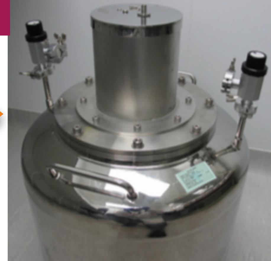
Potential component emanates radon in chamber (10 days+)
