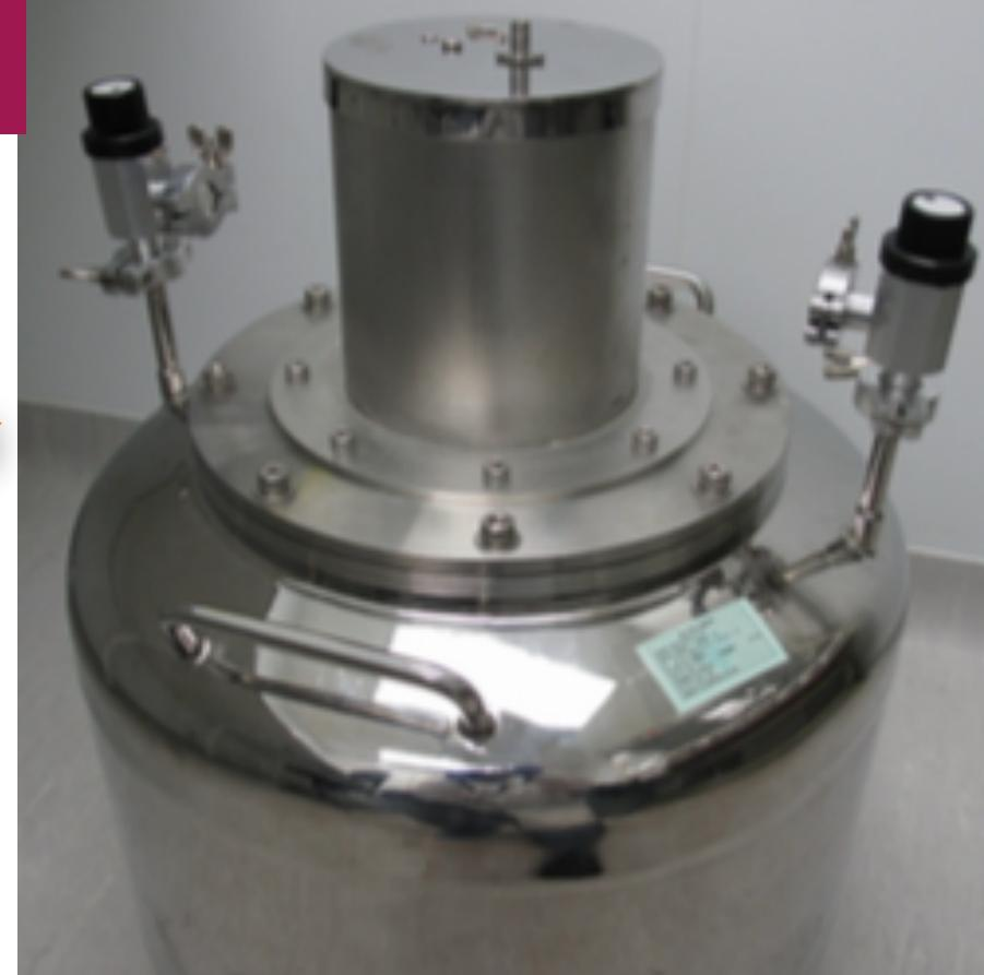
**70-litre** electrostatic detector can measure activities down to **0.09 mBq**
