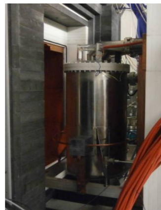
XENON100 Total Xe: 162 kg Target: 62 kg Fiducial: 34/48 kg Limit: \sim 10^{-45}
