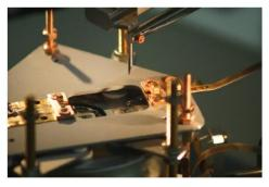
New signal and HV contacting by wire bonding flat ribbon cables
