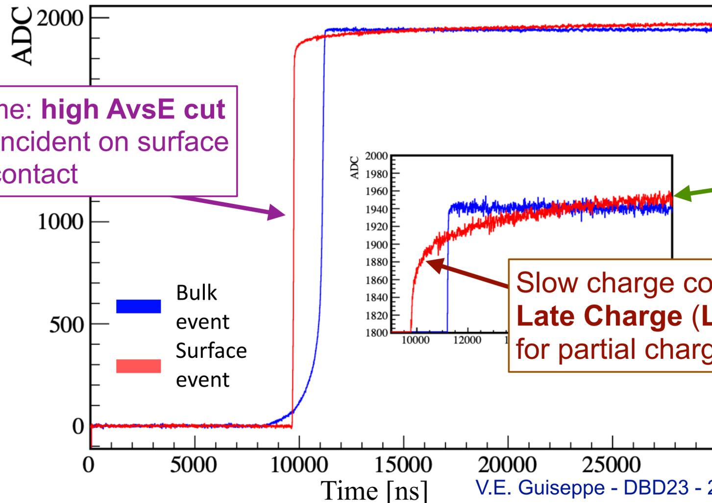
Fast drift time: **high AvsE cut** for particle incident on surface near point contact
