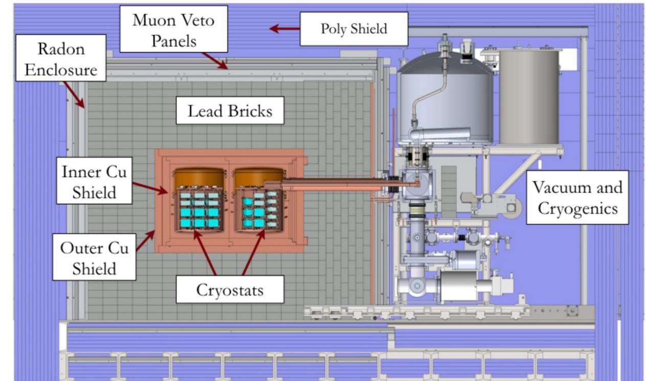
Continuing to operate at the Sanford Underground Research Facility with natural detectors for a  $^{180\text{m}}\text{Ta}$  decay search
