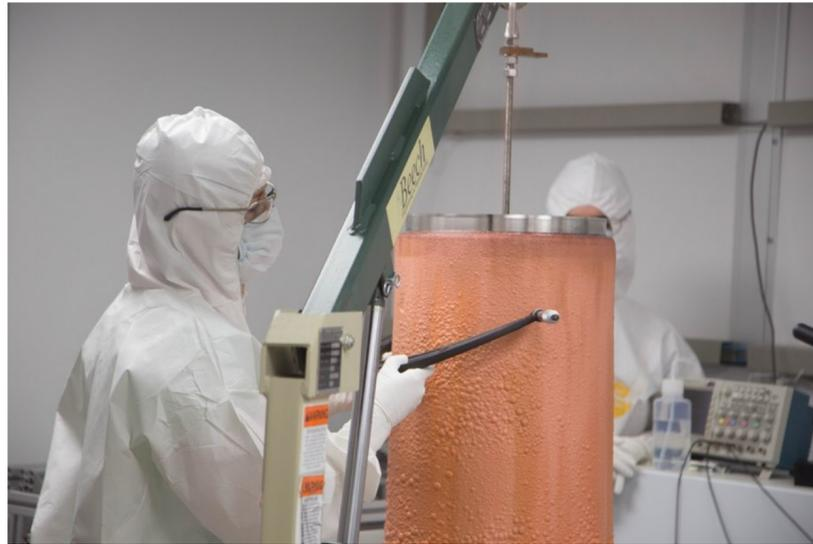
In-house production of underground electroformed Cu
