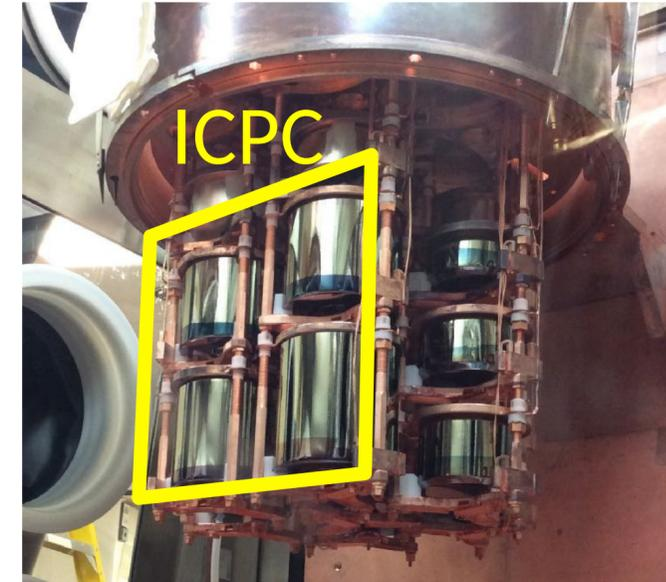
**Low Background:** 2 modules within a compact graded shield and active muon veto using ultra-clean materials
