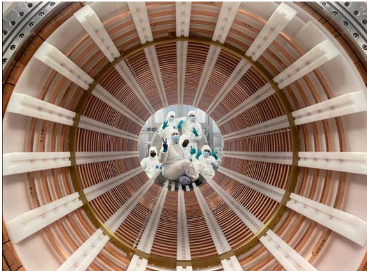
Field cage interior with transparent cathode
