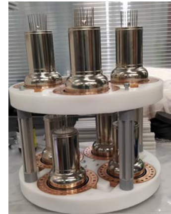
PMT energy plane installation with sapphire pressure windows in final stages
