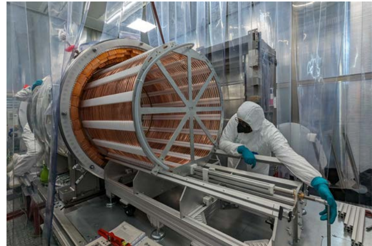
Teflon reflector panels with TPB
