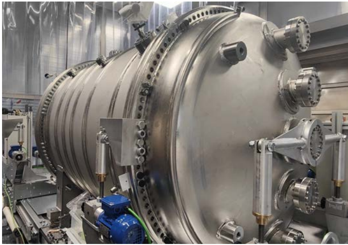
Stainless-steel pressure vessel + lead castle for shielding
