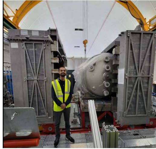
Stainless-steel pressure vessel + lead castle for shielding
